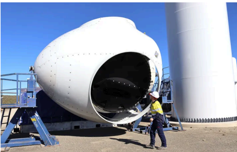
The rotor hub of a wind turbine at Brandvalley Wind Farm. The rotor hub holds the blades and connects them to the main shaft of the wind turbine. (Photo: Tamsin Metelerkamp)
